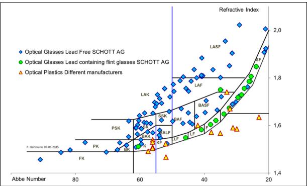
Fig. 1: Abbe-Diagram of optical plastics and optical glass
